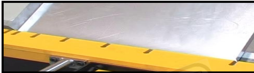
Folding a tray note that the folded sides fit into the slots
